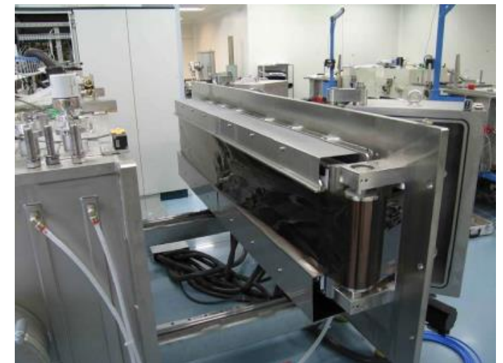
Deposition of the absorption layer (CIGS)
