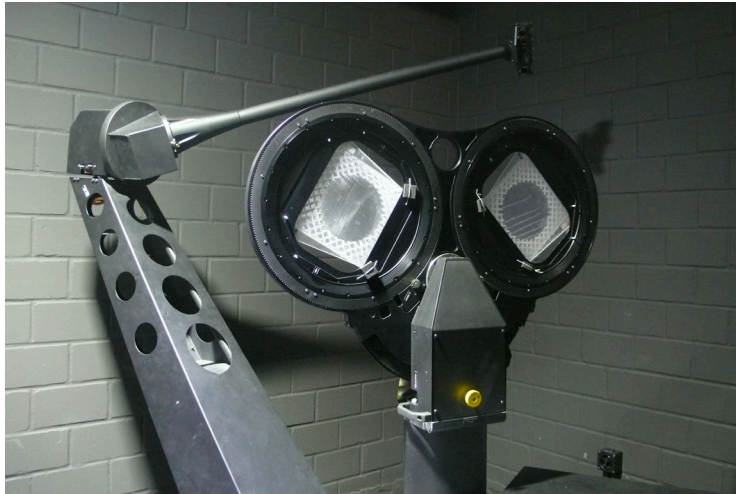
Goniophotometer Laboratory, Research Group Envelopes and Solar Energy, HSLU © Lars Grobe
