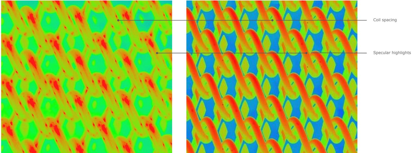
Comparisons between HDR photograph of the physical sample (left) and Radiance simulated mesh (right) under similar conditions
