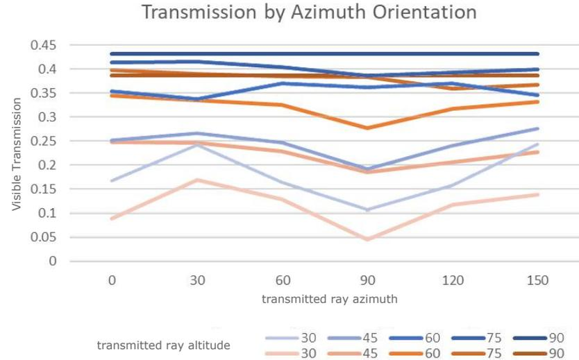
Comparisons between the angular VLT of the measured physical sample (in orange) and the simulated metal mesh (in blue) at 30 different altitude / azimuth angles.
