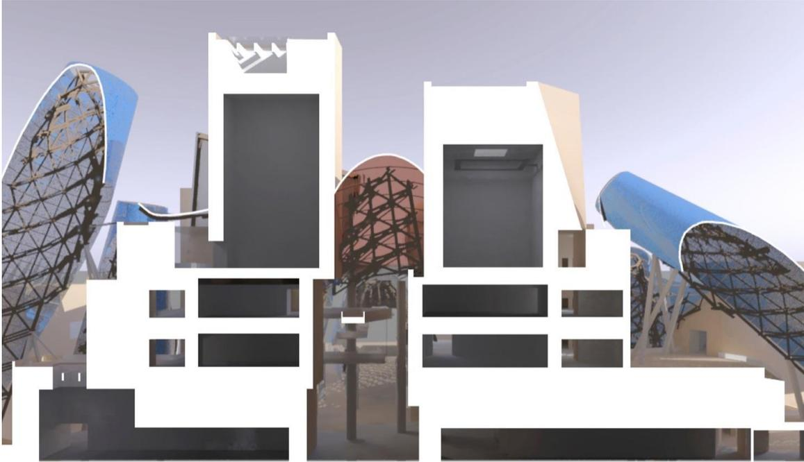
Section through atrium, cones, and galleries from daylight studies done in 2010. At that time the cones were glass with blue ceramic frit.
