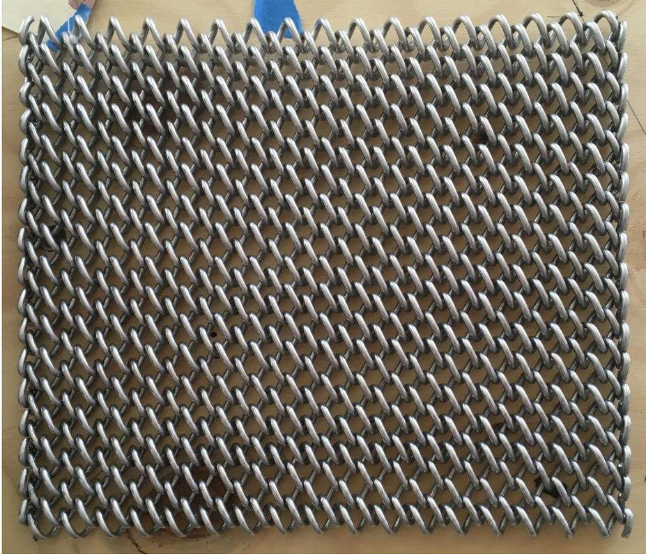
L+U had samples of a 9 gauge specular aluminum mesh and a 6 gauge galvanized steel mesh.
