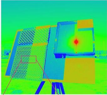
Specular reflections off of glass panels are intense, but angularly dependent and of limited duration. At the same sun and view angles, reflections from metal mesh are less extreme, but will remain for longer
