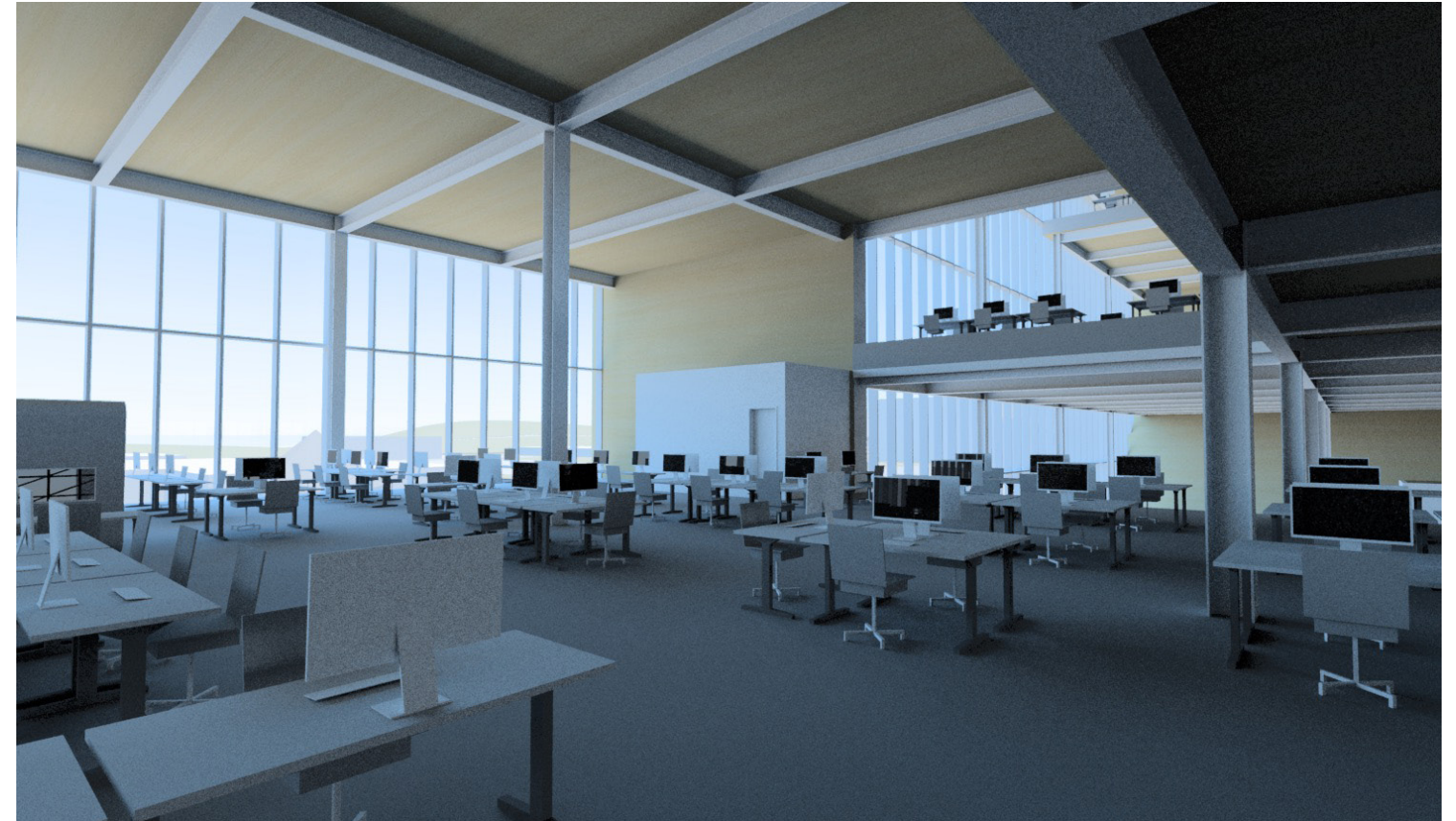
pcond -h -v- with sRGB primaries specified, modified to use E illuminant xr .64 yr .33 xg .30 yg .60 xb .15 yb .06 xw .333 yw .333 (pcond -h -v- -p .64 .33 .30 .60 .15 .06 .333 .333)
