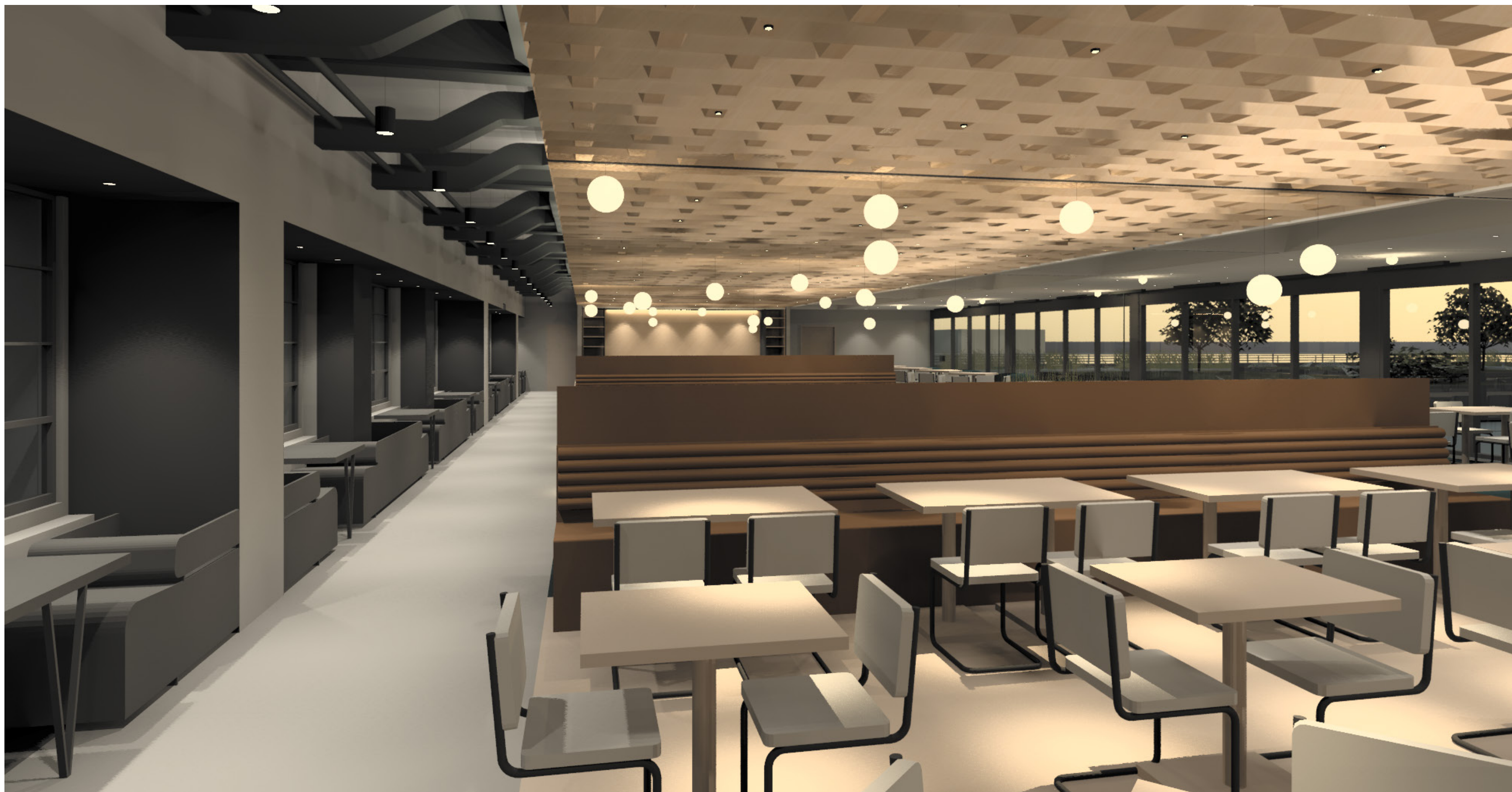
High-turbidity dusk Utah Sky used in electric lighting integration simulation when sky will have little to no interior contribution.
