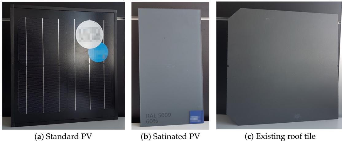
**Figure 7.** Photographs of material samples used in the case study: standard PV (a), satinated PV (b), and existing roof tile (c).
