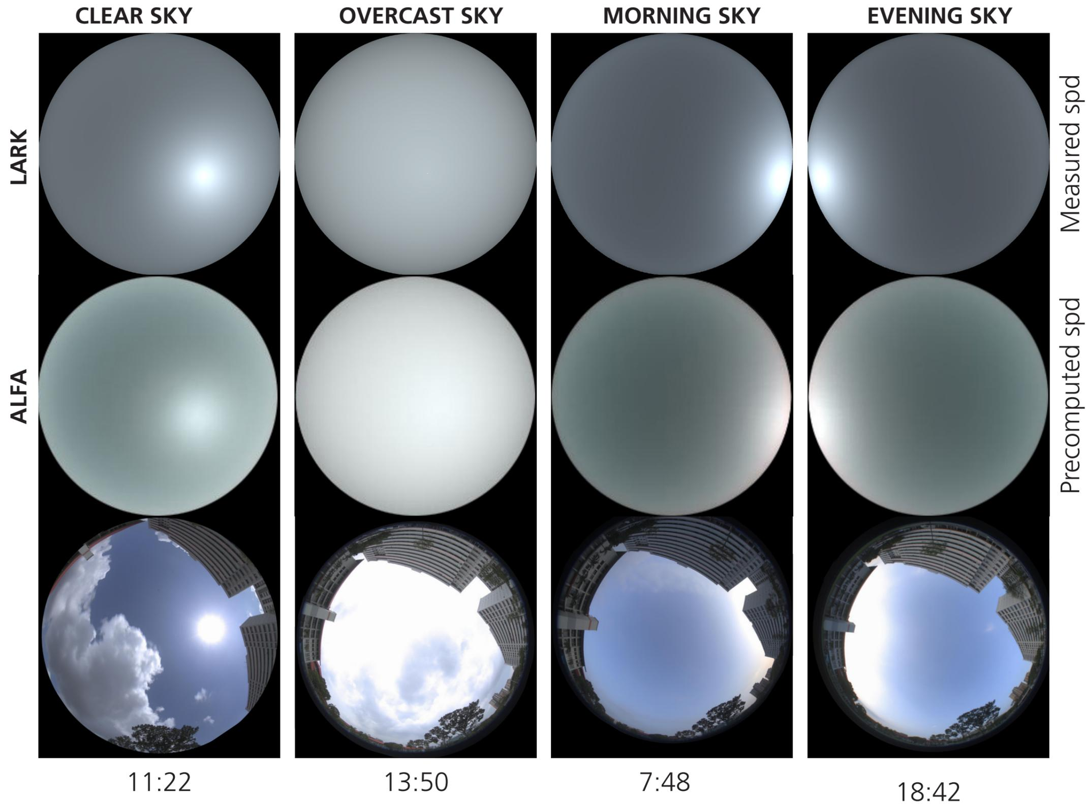
Lark uses measured global spectral irradiance and ALFA uses precomputed skies.
