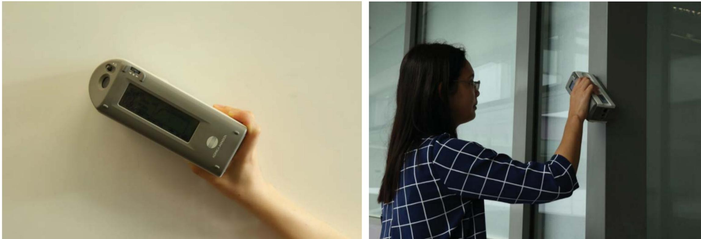
Konica Minolta 2600d spectrophotometer to measure spectral reflectance of materials
