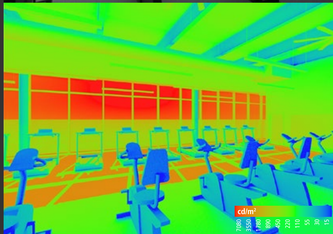
Falsecolor Luminance Map, Surface Brightness
