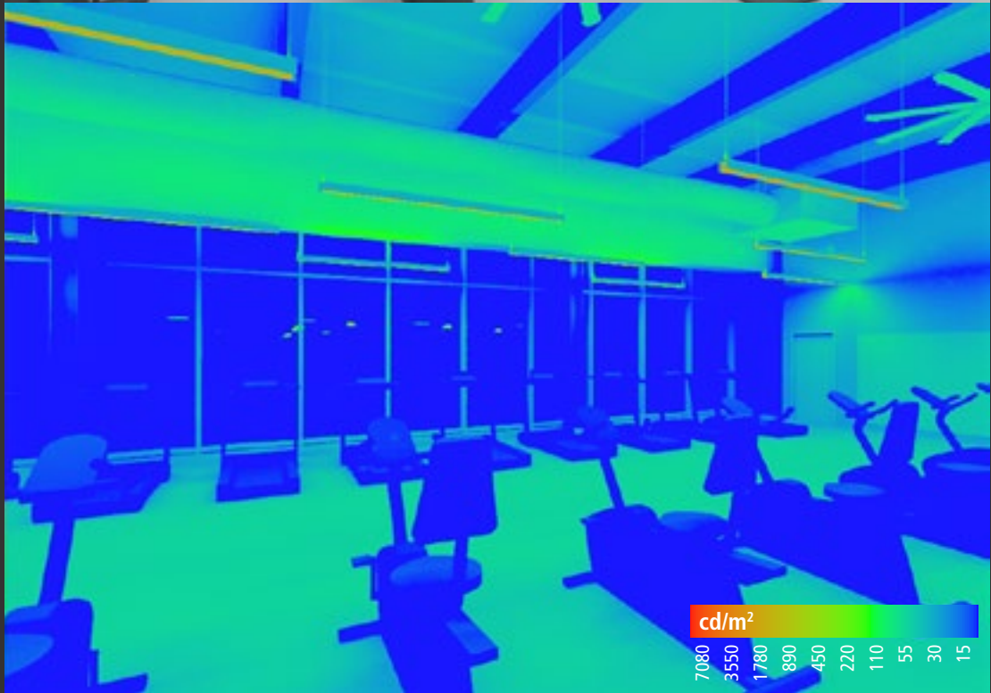
Falsecolor Luminance Map, Surface Brightness
