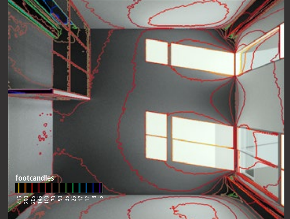
Plan Perspective - Daylight Illuminance Levels
