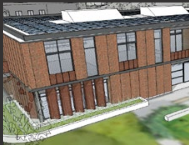
Exterior Automated Blinds
