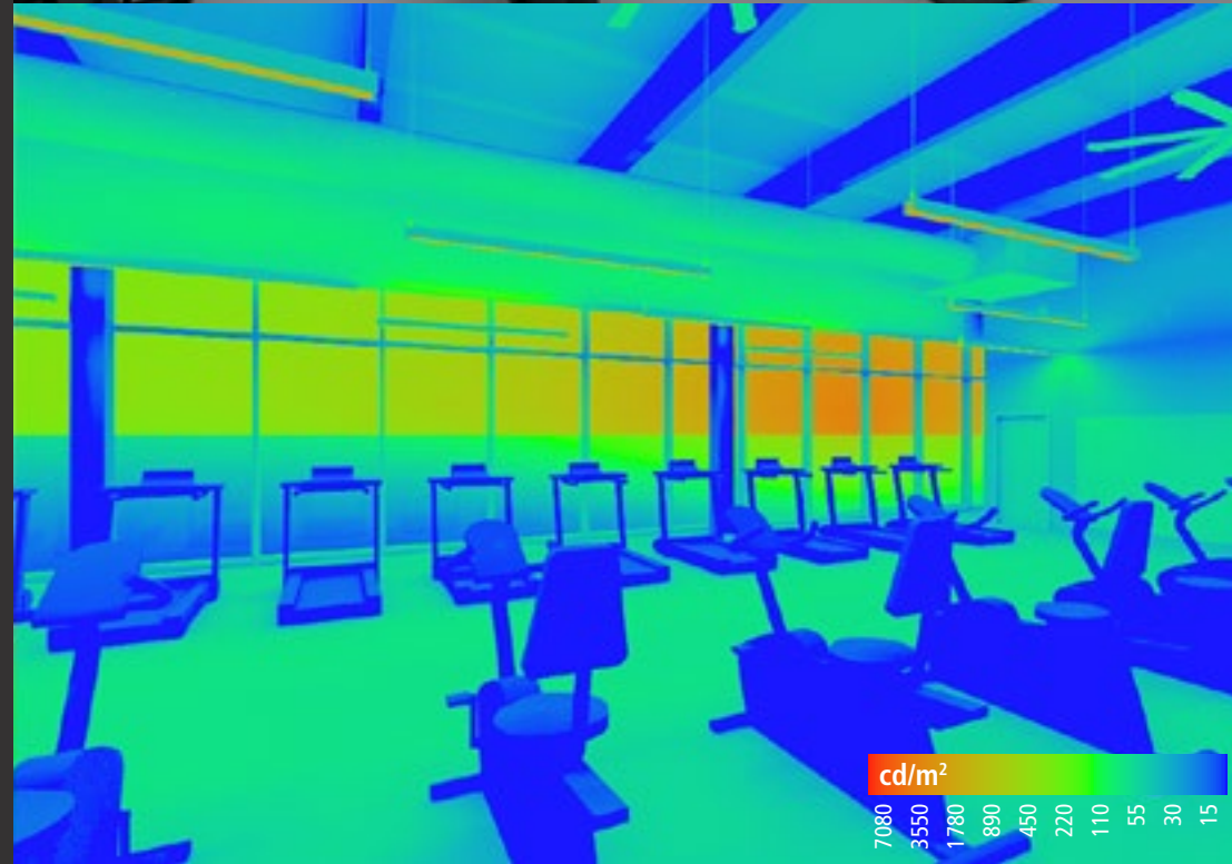
Falsecolor Luminance Map, Surface Brightness
