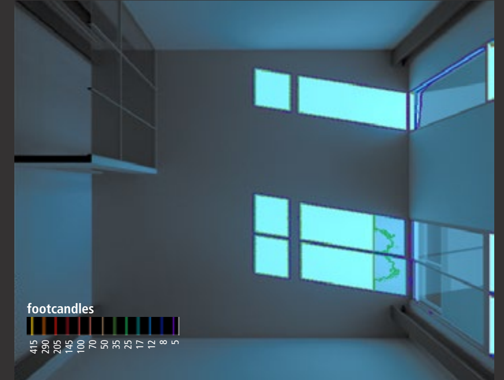
Plan Perspective - Daylight Illuminance Levels
