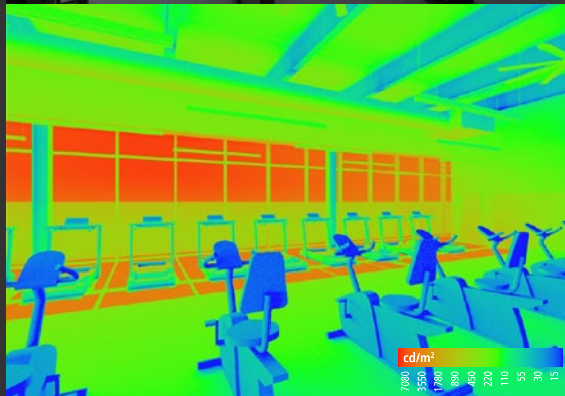
Falsecolor Luminance Map, Surface Brightness
