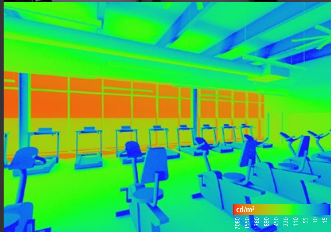
Falsecolor Luminance Map, Surface Brightness
