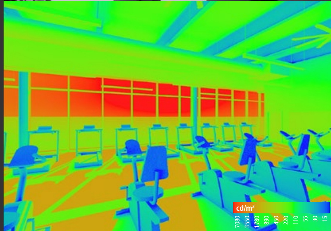
Falsecolor Luminance Map, Surface Brightness
