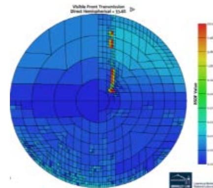
7 variable resolution BSDF for light-redirecting system
