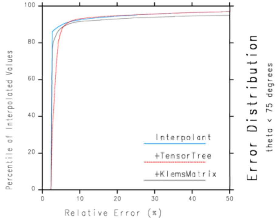
Error population of BRDF interpolant and tensor tree and Klems representations for 150M incident and exiting test direction pairs based on anisotropic Ward-Geisler-Moroder-Dür BRDF model (reference).
