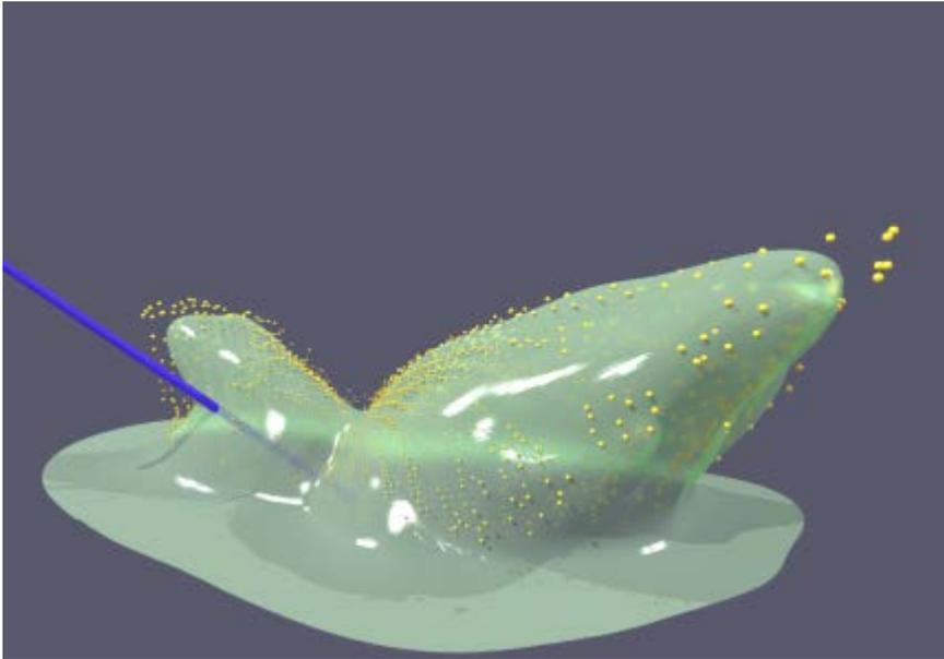
Interpolation of measured scattering values for a single incident direction, shown as blue line. Yellow dots are measurements, and green surface is interpolation using radial basis functions.
