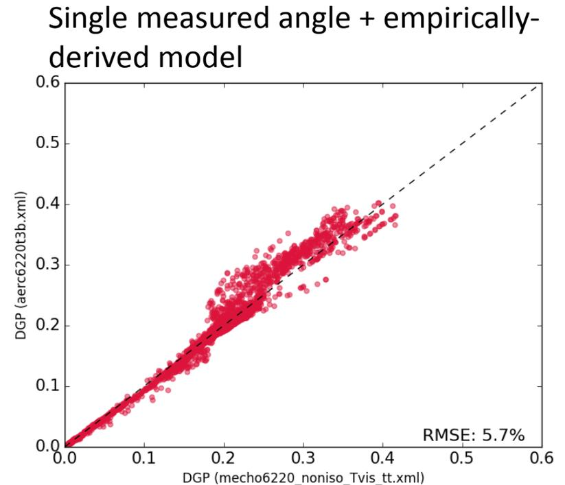
DGP computed using gold standard BSDF data (x-axis) versus alternate BSDF data (both modeled with 5-phase approach and high-resolution tensor tree format)
