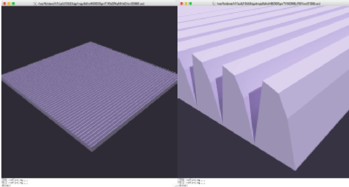
Figure 15 - screenshots of rvtv window displaying the prism model (with dielectric material replaced by blue plastic so prisms are visible).
