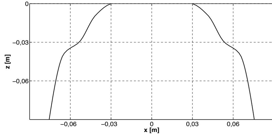
The figure of a tri-curve reflector profile calculated with the algorithm without constraints
