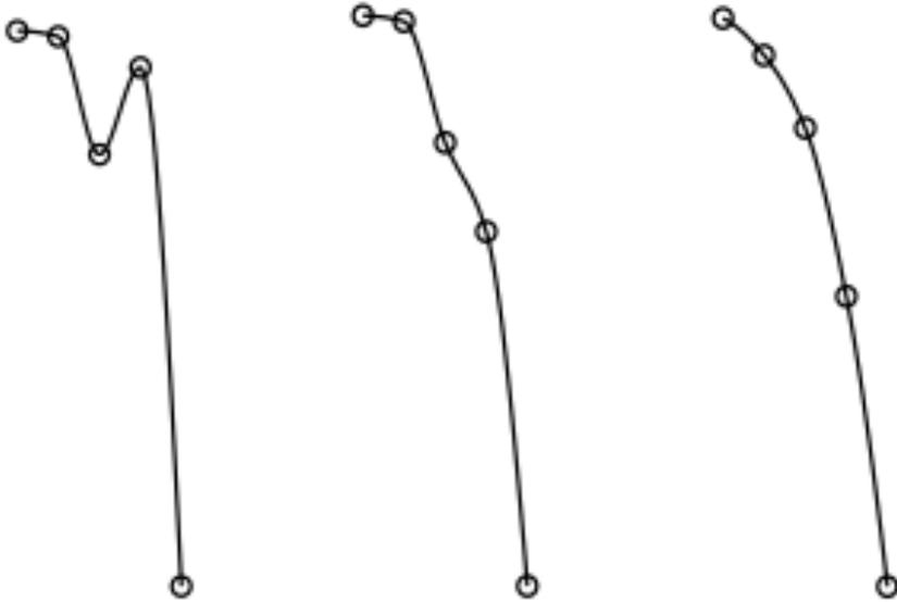
Reflector profile curves generated in the unconstrained optimisation process in the 3rd, 10th and 50th iteration
