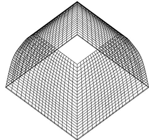
The reflector profile is described by the Hermite interpolating polynomial
