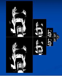
Grayscale images are scaled down repeatedly to create an image pyramid, which is then converted into MTBs for comparison
