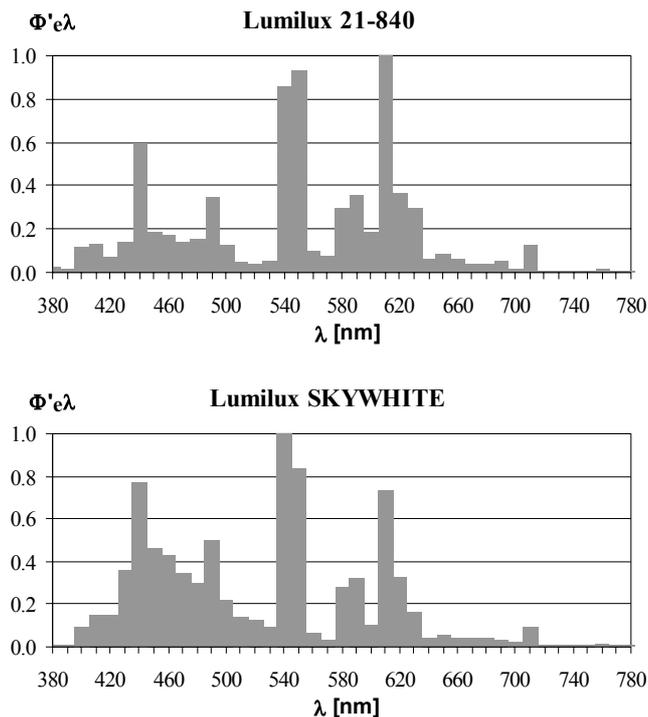
Fig. 3. Spectral distribution of the fluorescent lamp Lumilux 21-840 and Lumilux Skywhite.
