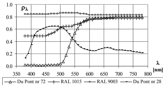
Fig. 4. Spectral reflectance factors of paints samples from Du Pont catalogue and coloured samples from RAL colours catalogue.
