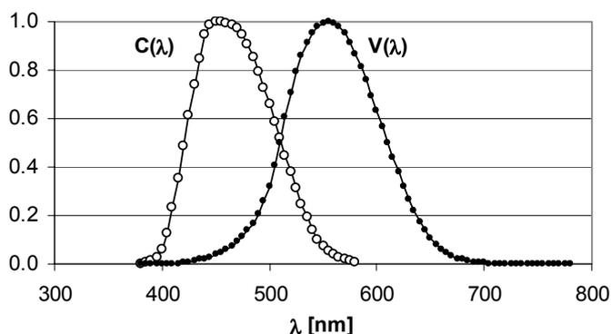
Fig. 1. The relative spectral luminous efficiency functions  $V(\lambda)$  and relative spectral circadian efficiency functions  $C(\lambda)$ .
