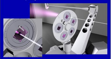
new: sample RFID, less self shadowing, larger samples
