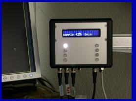
standard detector head (shielded, max 5 sensors)
