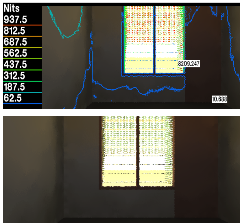
Figure 6a and 6b. Iso Contour Image and Luminance Image of Shiny Leaves 50% Porosity Full-Covered Vegetative Shading
