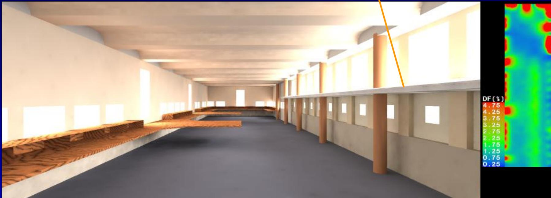
Inset shows plan view of daylight factor at work plane height
