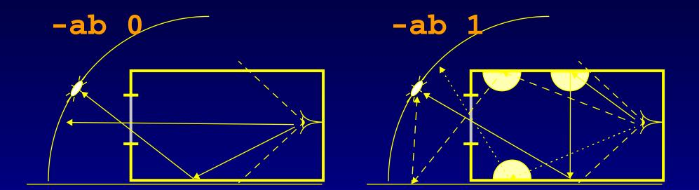
With the ambient calculation switched off, we see the sky (glow) through the window and whatever sun patches are directly visible from the view point.
