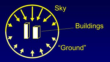
the sky and the ground will not affect the brightness of either. In other words, no matter how built-up the model becomes, with nearby tall structures and so on, the ground radiance (where it is visible) will be the same as for an empty scene. Therefore, all scenes should include a local ground plane that participates in the inter-reflection calculation.
