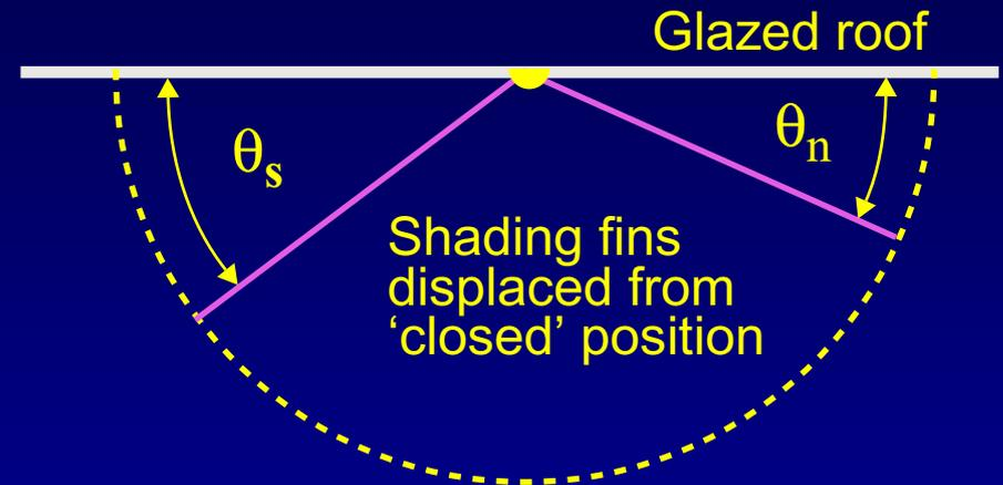
A slightly different scheme was used to displace fins on the other side of the hinge to introduce overall North-South asymmetry into the structure.
