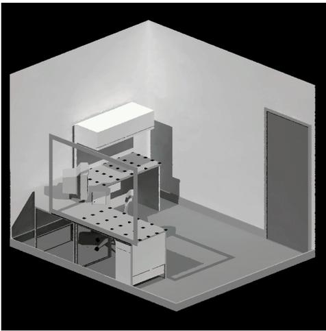
**Figure 3** Room configuration. The positions of the 50 work-plane points are represented by black squares on the desk surface. The window frame shows the position of the window.
