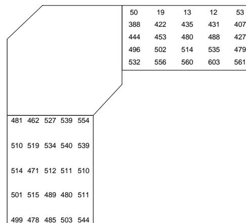
**Figure 6** Illuminance (lx) on the work planes obtained with the optimal luminous intensity distribution from the window.
