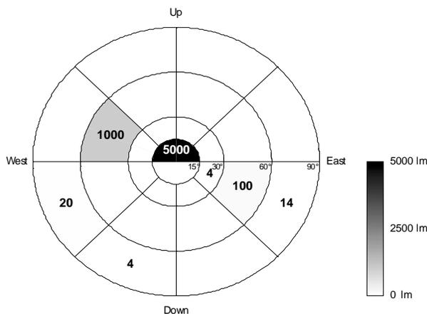
**Figure 5** Optimal luminous intensity distribution, showing flux emitted into each solid angle.
