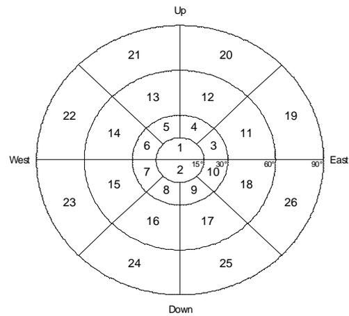
**Figure 4** Solid angle discretization.
