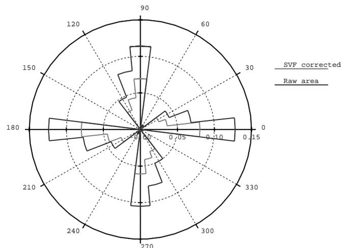
Figure 5: Polar diagram of the overall building facades of the urban site (raw area and Sky View Factor corrected)
