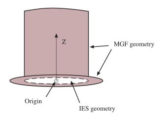
**Figure 3.** Geometric representation of can downlight fixture, and placement of IES simple geometry.
