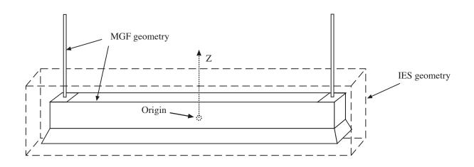
**Figure 4.** A hanging direct/indirect fixture and the surrounding IES simple geometry.
