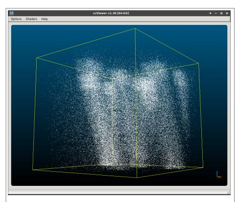
Figure 12: ASCII point list imported into an interactive point cloud processor/viewer (in this case *ccViewer*, part of the excellent open-source *Cloud-Compare* toolsuite [CC2020]). The point list was exported by *pmapdump* with the **-a** option from the volume map rendered in Figure 11.
