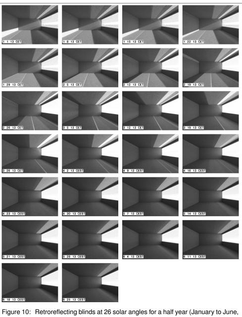
Figure 10: Retroreflecting blinds at 26 solar angles for a half year (January to June, in weekly intervals) rendered with contribution photon map and *rcontrib*. In each instance the time of day is 1:00pm. Redirection and transmission dominate until March, while retroreflection dominates in the following months.
