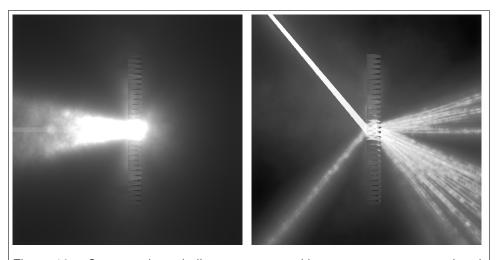
Figure 16: Compound parabolic concentrator with opaque apertures rendered with volume photon map in a *mist* environment. At normal incidence (left), the incident beam is retroreflected, whereas at  $50^{\circ}$  incidence (right) it is transmitted and redirected in a characteristic fan-out.
