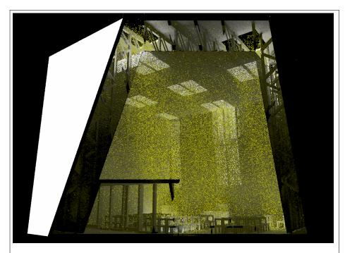
Figure 11: Cutaway view of volume photons entering a modernist church through skylights, rendered with default *pmapdump* output (yellow spheres) merged with the original scene geometry. Model courtesy of Prof. Nozomu Yoshizawa, Tokyo University of Science.
