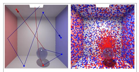
Figure 2: Global photon distribution in the Cornell box. Left: global and caustic photon paths during forward pass. Dots indicate stored photons, where blue represents global photons, and red represents caustic photons. Right: photon distribution after completion of forward pass (visualised with *pmapdump*). Note the concentration of caustic photons on the back wall reflected from the glass sphere.
