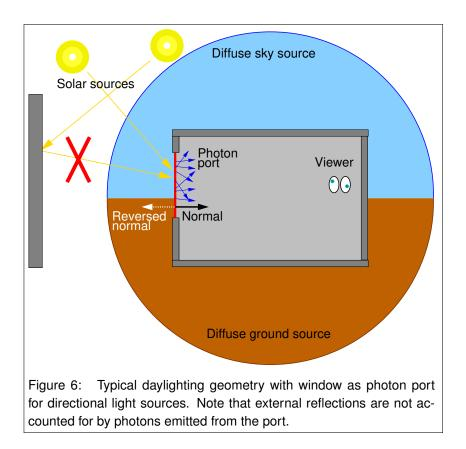
In addition, ports can also be configured to emit bidirectionally, i.e. from either side. A possible use case is using a *mist* volume boundary as port; per definition, the photon will only scatter if it enters the medium, i.e. if its normal points outwards. In this case, the port needs to be reoriented to face inwards.
