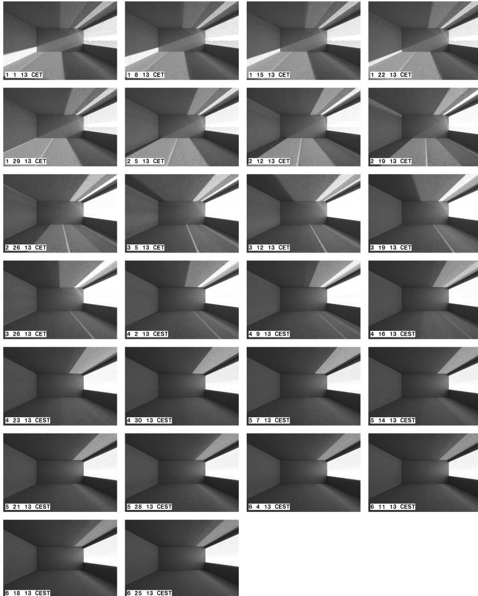
Figure 9: Retroreflecting blinds at 26 solar angles for a half year (January to June with weekly intervals) rendered with contribution photon map and *rcontrib*. In each instance the time of day is 1:00pm. Redirection and transmission dominate until March, while retroreflection dominates in the following months.
