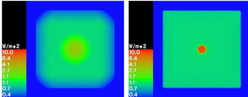
Figure 5: Left: falsecolour rendering of severely biased caustic with a bandwidth of 5000 photons. The caustic should have an irradiance of  $10 W/m^2$ . Right: falsecolour rendering of the same caustic with bias compensation using a bandwidth of 50–5000 photons.
