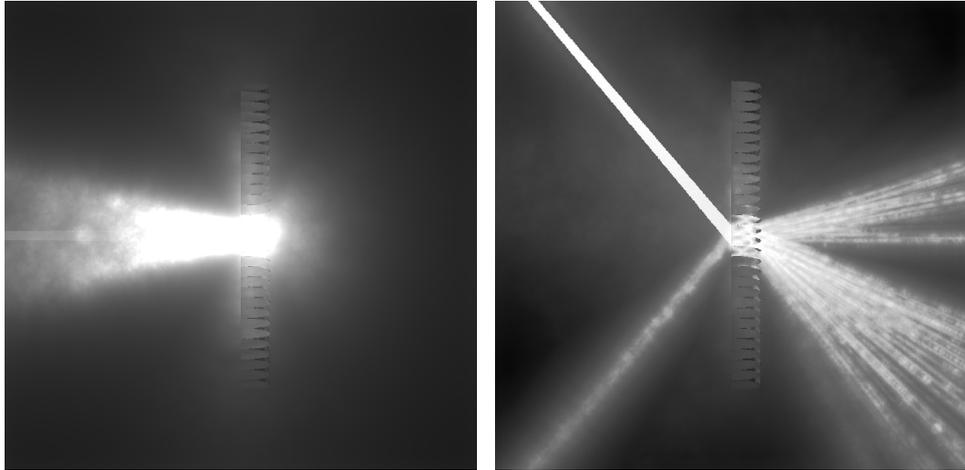
Figure 12: Compound parabolic concentrator with opaque apertures rendered with volume photon map in a *mist* environment. At normal incidence (left), the incident beam is retroreflected, whereas at  $50^\circ$  incidence (right) it is transmitted and redirected in a characteristic fan-out.
