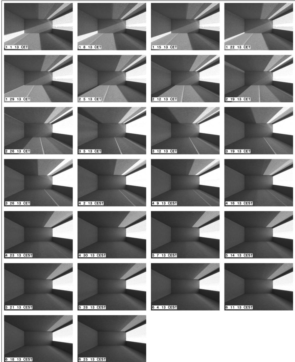
Figure 10: Retroreflecting blinds at 26 solar angles for a half year (January to June, in weekly intervals) rendered with contribution photon map and *rcontrib*. In each instance the time of day is 1:00pm. Redirection and transmission dominate until March, while retroreflection dominates in the following months.
