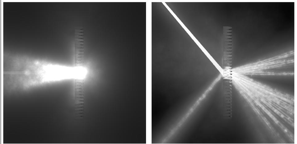
Figure 16: Compound parabolic concentrator with opaque apertures rendered with volume photon map in a *mist* environment. At normal incidence (left), the incident beam is retroreflected, whereas at  $50^\circ$  incidence (right) it is transmitted and redirected in a characteristic fan-out.
