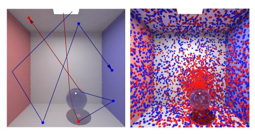
Figure 2: Global photon distribution in the Cornell box. Left: global and caustic photon paths during forward pass. Dots indicate stored photons, where blue represents global photons, and red represents caustic photons. Right: photon distribution after completion of forward pass. Note the concentration of caustic photons on the back wall reflected from the glass sphere.
