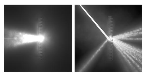
Figure 12: Compound parabolic concentrator with opaque apertures rendered with volume photon map in a *mist* environment. At normal incidence (left), the incident beam is retroreflected, whereas at  $50^{\circ}$  incidence (right) it is transmitted and redirected in a characteristic fan-out.
