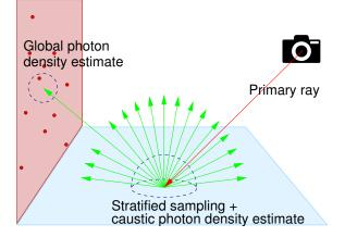
Figure 8: Caustic photons are visualised at the primary ray, while an intermediate stratified sampling step is used between the primary ray and the global photon density estimate (*final gather*).
