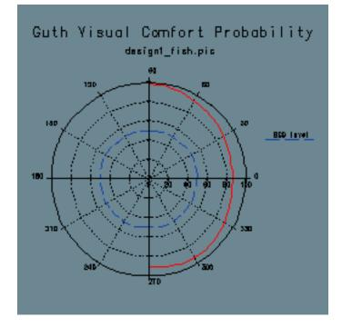
**Figure 8b.** Visual comfort probability (VCP, glare) calculation for cubicle office space, showing a numerical plot of VCP. The zero degree view is looking straight ahead in the image shown, and positive angles look to the right. A VCP of 75% means 75% of occupants are comfortable.
