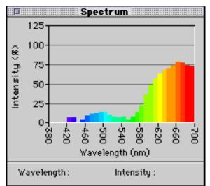
Figure 2. Spectral reflectance measurement from Colortron<sup>™</sup> spectrometer. Each waveband is about 10 nm wide.
