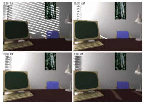
Figure 10. Four frames from a time-lapse animation of a small office with venetian blinds, computed by *Radiance*.
