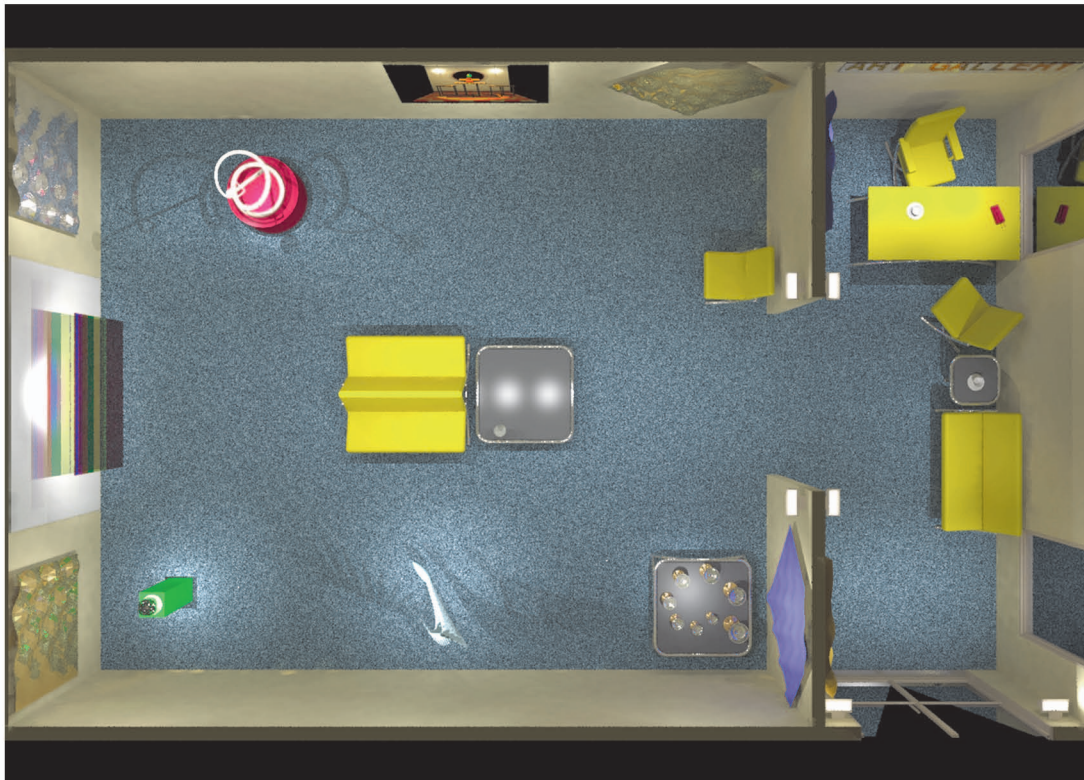
Plate 14 A plan view ( scene_na.pic ) of the gallery reveals pools of light around each sculpture. The tracklights draw attention to the art and add to the visual interest of the room. (See also Figure 3.48 on page 225.)
