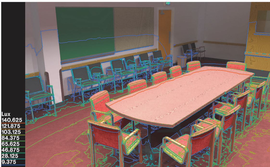
Plate 3 A simulation of the conference room with superimposed isolux contours (i.e., lines of equal illuminance). This emphasizes the numerical nature of the results, showing information that is critical for lighting analysis.
