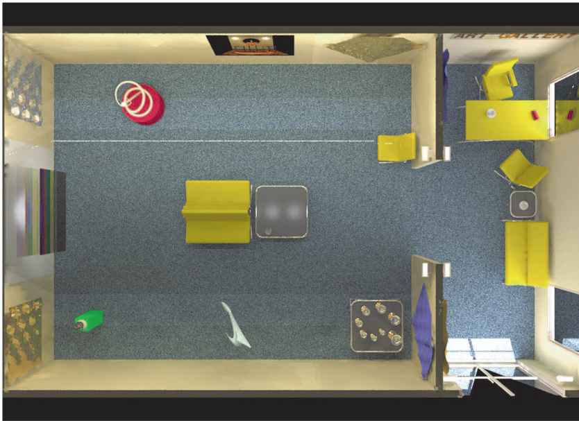
Plate 13 Picture scene2_da.pic presents a plan view of the day-lighted scene. Note the patch of direct sunlight on the carpet by the front doors and the line of sunlight in the gallery, which has slipped past the edge of the skylight reflector. The lobby desk and chair are illuminated from the sky components; the art in the gallery is lighted by indirect daylight. (See also Figure 3.46 on page 222.)
